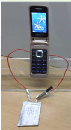
IITB battery is powering a mobile phone
