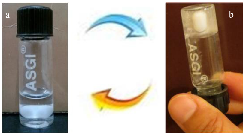
Figure 3. Photographs of the vial containing the colloidal suspension and a teflon coated magnetic pellet at (a) T > 60^{\circ}\text{C} and (b) RT
