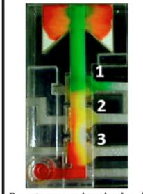
Paper to paper valves developed by Dr. Bhushan Toley. Valves 1,2 and 3 can be used for sequential delivery of different fluids.
