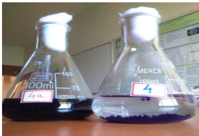
Figure 3: Comparison between untreated dye sample [A] and treated dye sample [B].
